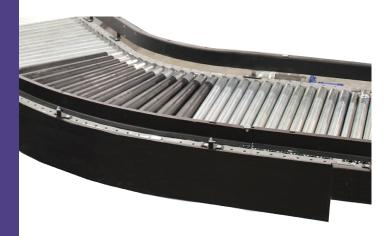
Automotion's Model CVB V-Belt driven conveyor incorporate a modular bolt together design enabling numerous job specific assemblies to be configured from a handful of standard modular components. These motor driven or slave driven units are available in a full array of curve, straight and junction configurations to satisfy your specific curve, merge, or divert layout requirements.
